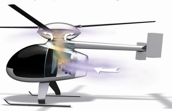
Flight safety: no tail rotor and capacity to overspeed the rotor in order to reduce the «dead man zone».
